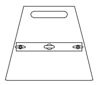
Single flybar allows one R2 to be suspended from a single point. Tilting and directional control can be affected using lines to the lower side fixing points.
